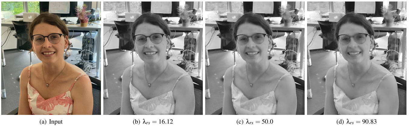
Figure 9: Input image and corresponding shading output with increasing value of threshold \lambda_{rs} . The “Retinex-Shading smoothness” term smooths the output shading while preserving the edges. However, if the smoothing is more it starts blurring important details, see (d).
